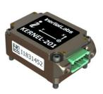
The Inertial Labs KERNEL-201 is a breakthrough, fully integrated inertial solution that combines the latest MEMS sensor technologies. Fully calibrated, temperature compensated, mathematically aligned to an orthogonal coordinate system, the IMU contains up to 0.7 deg/hr Bias inrun stability gyroscopes and 0.005 mg Bias inrun stability accelerometers with up to ±40 g dynamic range, very low noise and high reliability.
