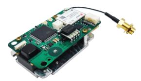
The Inertial Labs **INS-U-OEM** utilizes advanced single antenna GNSS receiver, two barometers, magnetometers, 3-axes each of calibrated in full operational temperature range Advanced MEMS Accelerometers and Gyroscopes to provide accurate Position, Velocity, Heading, Pitch and Roll of the device under measure.
